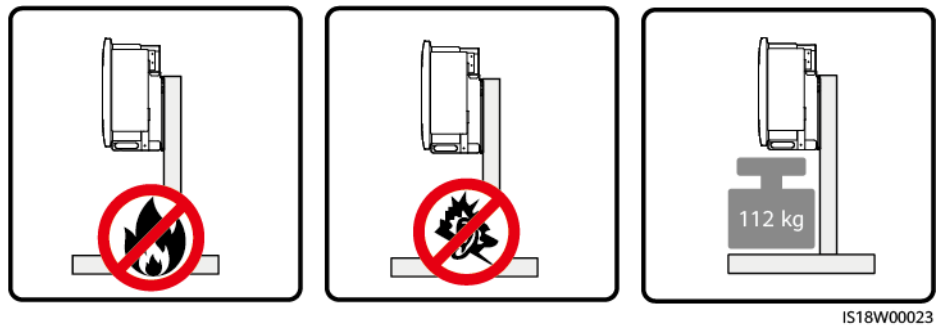
Figure 4-2 Mounting structure requirements
